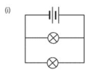
(j) When bulbs are connected in parallel, the overall resistance of the circuit is reduced. Both bulbs would glow with equal brightness but more brightly than in the series circuit.
